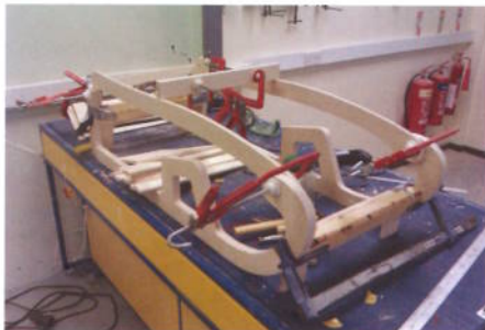
Figure 5 Assembly of wooden frame
